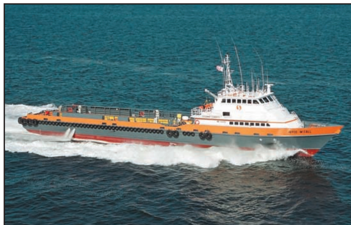
The crew boat Joyce McCall is powered by four KTA50-M2 engines
